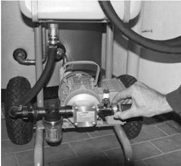
1. Connect filling hose to pump outlet.
