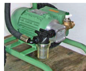
filter ahead of and pressure relieve valve behind the pump
