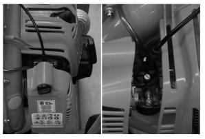
Clean filter with a non inflammable cleaning liquid (for example luke warm soap solution) and dry it.
